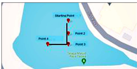
Figure 7. Movement of the autonomous floating net cage based on water quality sensor readings
