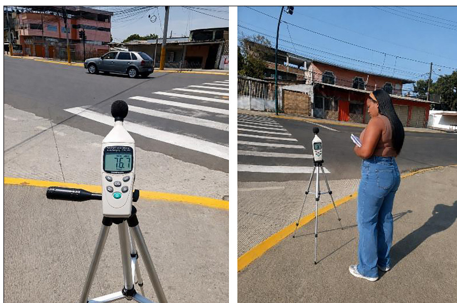
Figure 2. Instrumental recording of acoustic monitoring in the field
