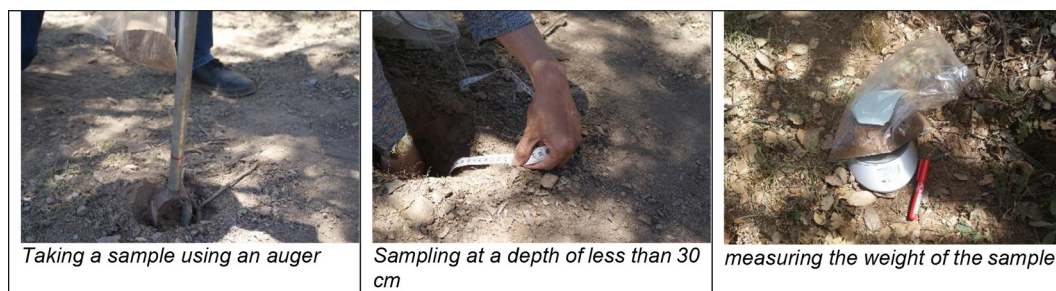
Figure 3. Photographs of the field sampling procedure
