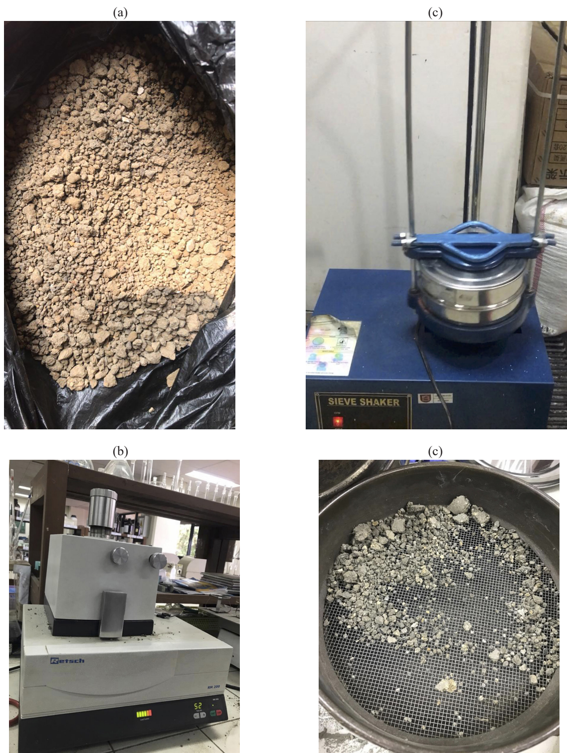
Figure 1. Soil sample preparation for remediation: (a) soil sample, (b) mortal grinder RM200, (c) sieve shaker
