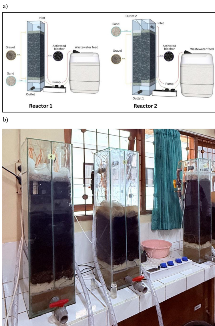
Figure 1. Laboratory-scale column filter reactor: (a) schematic illustration of internal layer configuration and flow path; (b) photograph of the assembled reactors during operation
