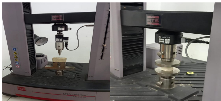
Figure 4. The mechanical tests using the MTS Criterion Model 43 machine, (a): The 3-point bending test, (b): The compression test
