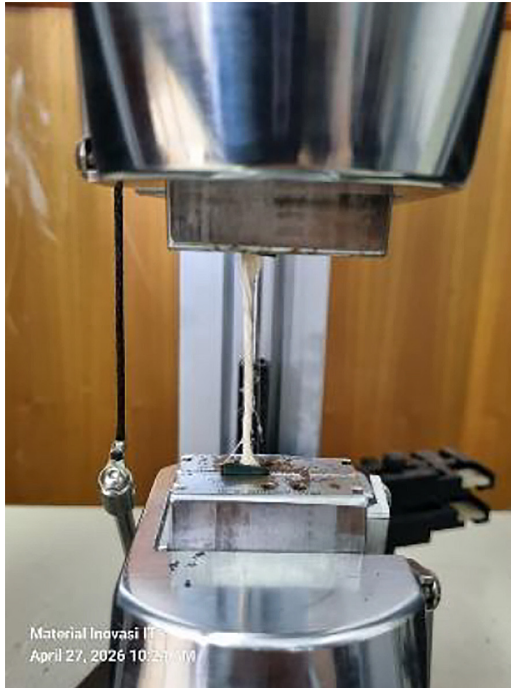
Figure 2. Tensile testing of Tamban pineapple leaf fiber bundles using a Universal Testing Machine (UTM)
