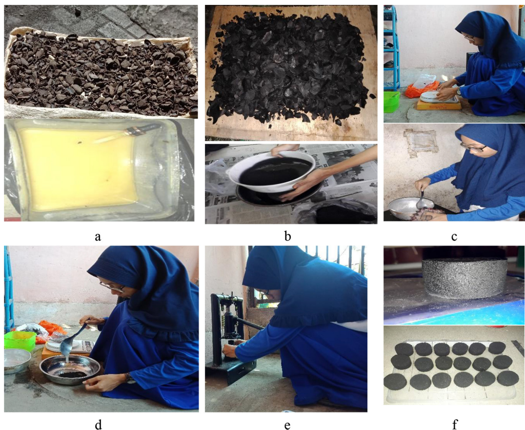
Figure 1. Experimental setup and briquette preparation process, (a) raw materials, including Pangium edule shell and pine resin, (b) Pangium edule shell charcoal, (c) preparation of cassava waste starch binder, (d) mixing of charcoal and binders, (e) briquette molding and pressing, and (f) drying process
