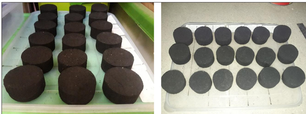
Figure 3. Physical appearance of Pangium edule shell charcoal briquettes produced under different binder formulations
