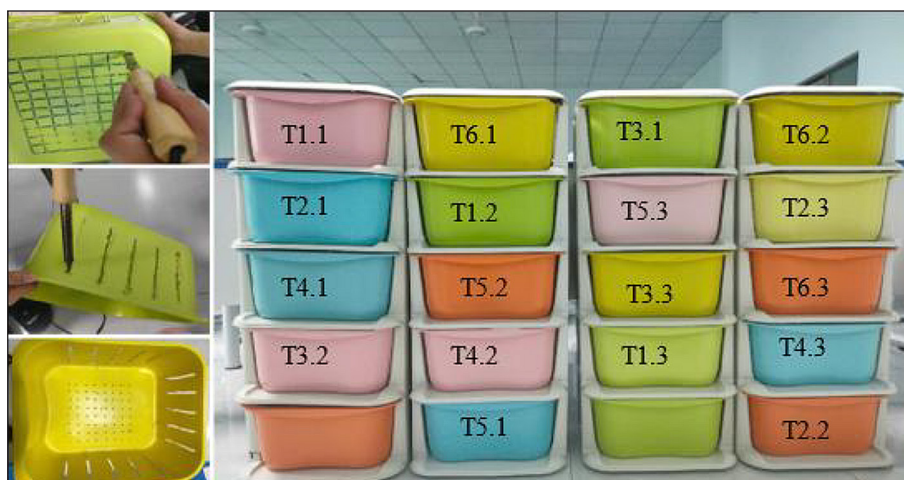
Figure 1. Laboratory-scale composting system and randomized allocation of the 18 experimental units according to the completely randomized design (CRD)
