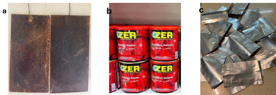
Figure 2. Electrode materials: (a) commercial mild steel electrode, (b) tomato paste cans, (c) recycled mild steel electrode
