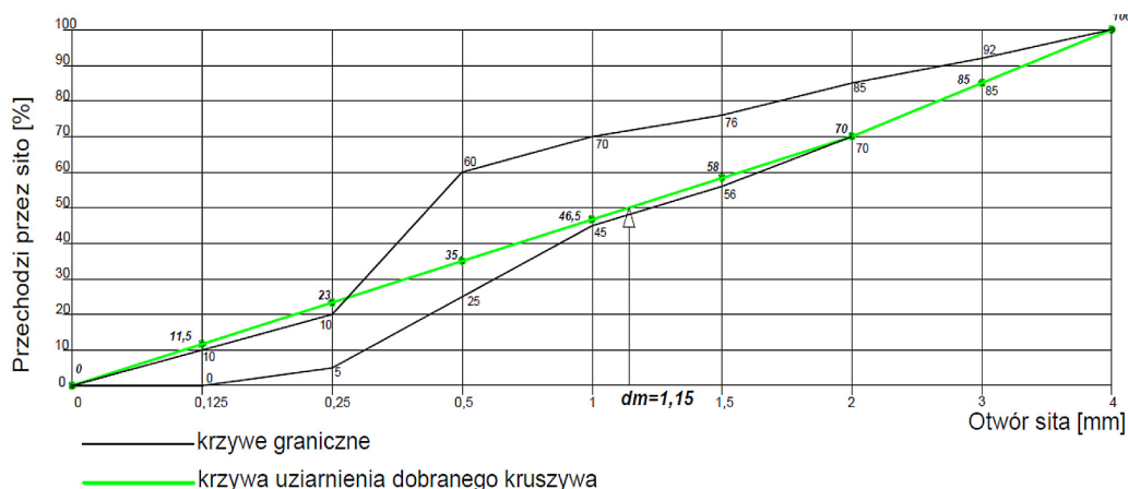
Rys. 1. Krzywa uziarnienia dobranej kruszywa Fig. 1. Grain size distribution curve for the selected aggregate
